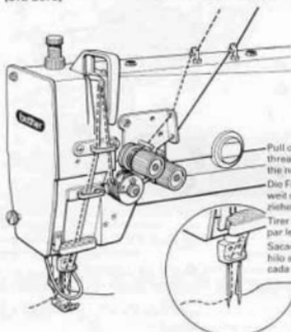
Pull out about 50 mm of thread through each of the needle eyes.
