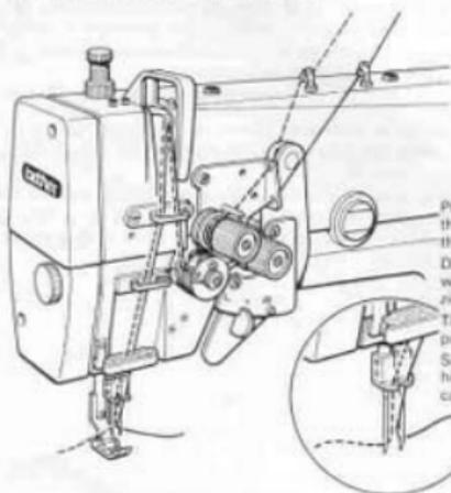
Pull out about 50 mm of thread through each of the needle eyes.
